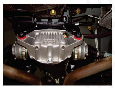
FIGURE 8: Bracket aligned and torqued
