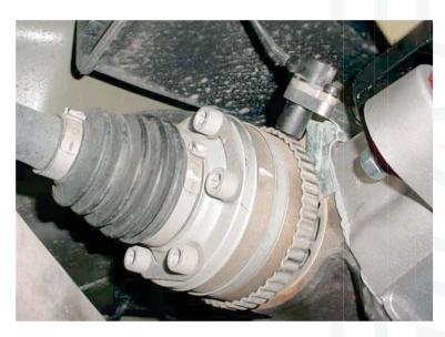
FIGURE 7: Set 1.0mm clearance between the sensor and reluctor
