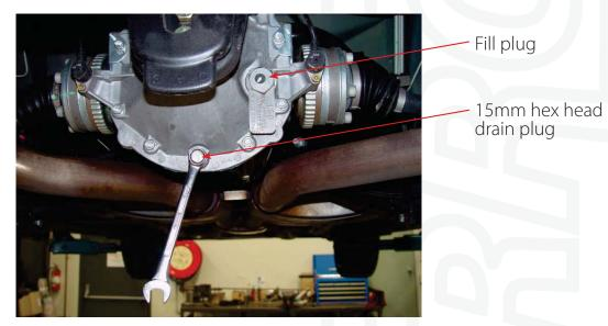
FIGURE 2: 15mm differential drain plug being removed
