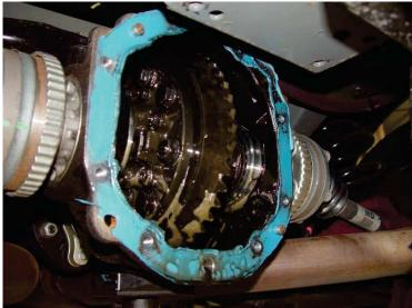
FIGURE 5: Clean the sealant from mating surface
