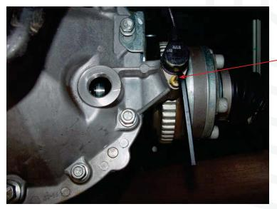
FIGURE 3: Removing the 2 speed sensors
