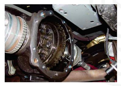
FIGURE 6: Once sealant is removed from mating face, begin reassembly
